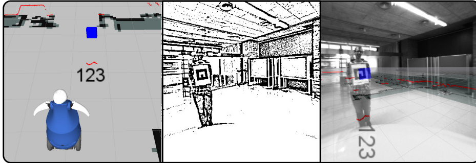
Figure 3.5: Combined laser (left) and marker detection (right: video image; centre: binarized image).
