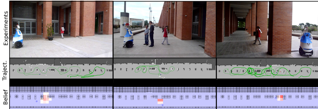
Figure 5.10: Top : Some scenes of the performed experiments in the BRL. Center : The trajectory during the experiments, indicated by the line. Bottom : The belief of the person’s location (red represents a high probability). Note that the maps are scaled differently.
